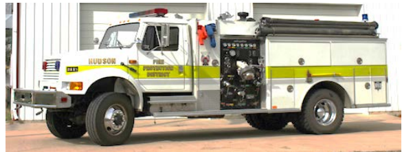
2835 Brush truck Year: 1991 1000 GPM pump; 750 Gallon tank
