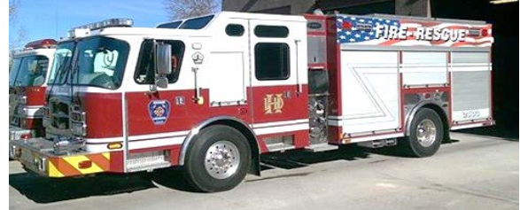
2803 Engine Year: 2012 1500 GPM pump 750 Gallon tank
