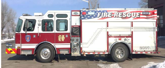
2801 Engine Year: 2013 1500 GPM pump 750 Gallon tank
