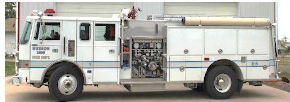
2813 Engine (Reserve – Station 3) Year: 1991 1000 GPM pump 1000 Gallon tank
