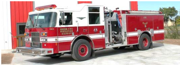
2811 Engine (Reserve – Station 1) Year: 2003 1260 GPM pump 750 Gallon tank
