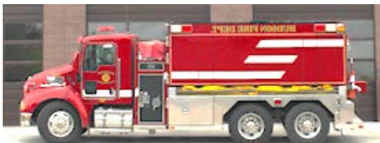
2841 Pumper/Tender Year: 2007 3000 Gallon tank 500 GPM pump
