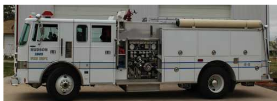
2805 Engine Year: 1991 1000 GPM pump; 1000 Gal tank
