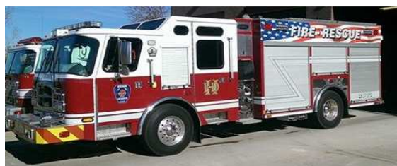
2803 Engine Year: 2012 1500 GPM pump; 750 Gal tank
