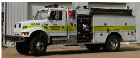
2801 Engine Year: 1991 1000 GPM pump; 750 Gal tank Pump & roll capabilities for wildland fires
