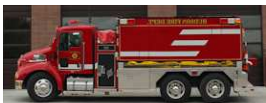
2842 Pumper/Tender Year: 2007 3000 Gal tank, 500 GPM pump
