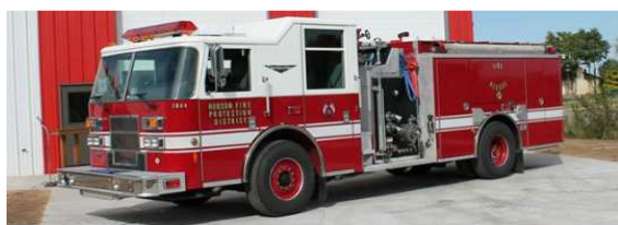
2804 Engine Year: 2003 1260 GPM pump; 750 Gal tank
